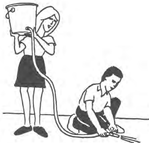
Fig 27 A simple demonstration of pressure - you can use it to understand the head of pressure concept.
