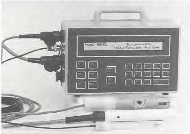
Fig 30 A field-lab analyser for conductivity, salinity, pH, temperature, dissolved oxygen. Illustration courtesy TPS Pty. Ltd. (Reproduced with permission)
