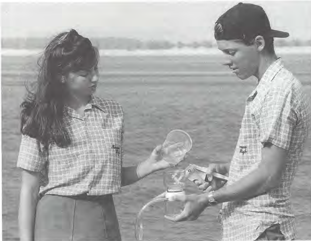
Fig 28 Using a membrane filter pad set, showing the two sections and the hand pump
