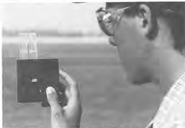
Fig 37 Hold the comparator up to the light and rotate the disc until you get a colour match.
