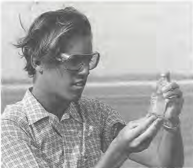
Fig 4 Dissolved oxygen bottle and sample
