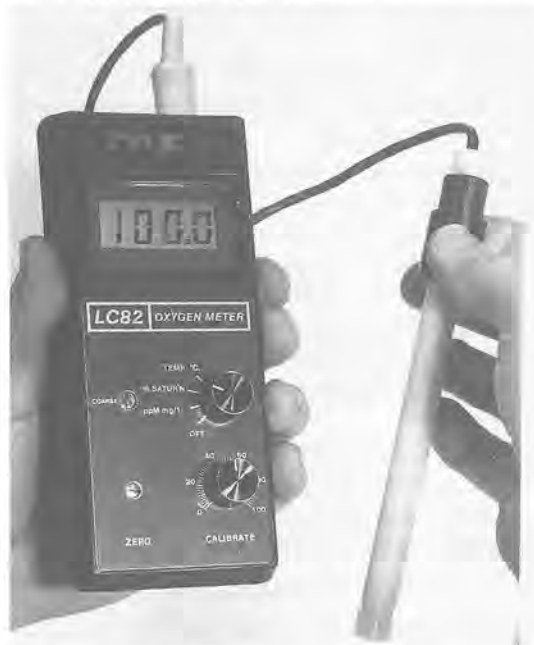
Fig 31 A dissolved oxygen meter. Illustration courtesy TPS Pty. Ltd. (Reproduced with permission)
