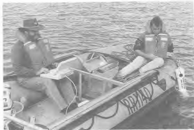
Fig 14 Water quality officers taking measurements of dissolved oxygen and temperature in a dam
